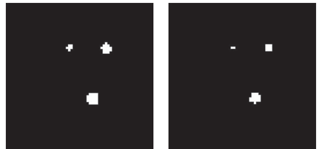
FIGURE 25.5 PPMs for two thresholds. Left: the default thresholds ( \gamma = 0 , p_T = 1 - 1/N ) Right: the thresholds \gamma = 0.3 , p_T = 0.95 .
